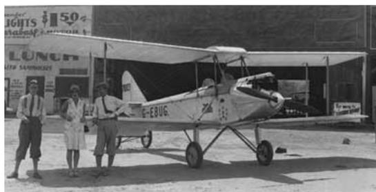
To appreciate the enormity of such a flight, one should read the specs for the aircraft: max speed: 102 mph; cruising speed: 87 mph; climb: 650 fpm; ceiling: 18,000 ft; gas capacity: 35 gal; max range: 400 miles. Aircraft length: 24'3"; height: 8'6"; wingspan: 28'; tare wt: 1130 lbs; max wt: 2002 lbs; present engine: Gypsy II, 120 hp.
