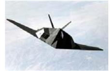
The design minimizes both radar and infrared signatures by using a combination of special materials, angles and shielded jet intakes and outlets. Its black exterior helps to hide it at night. The first flight was made in 1981. 54 aircraft were built for the USAF.
