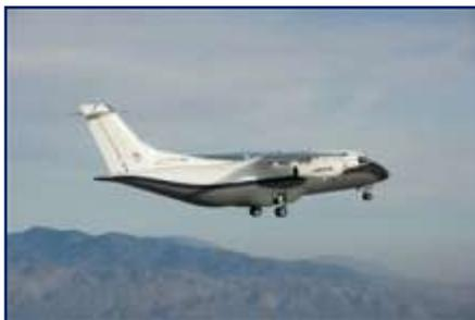
first test flight June 2 from Air Force Plant 42 in Palmdale, Calif. The ACCA is proof of concept technology demonstrator for advanced composite manufacturing processes in a full-scale, certified aircraft. It was developed by the Air Force Research Laboratory and Lockheed Martin.
